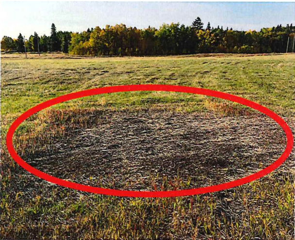
Above - Hay field showing dead grass area and extreme arid soil - indicating gas leak area
